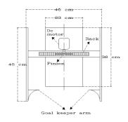
Fig.2. Sliding arm movement
